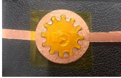
Figure 29. Completed production of DBD ion thruster
