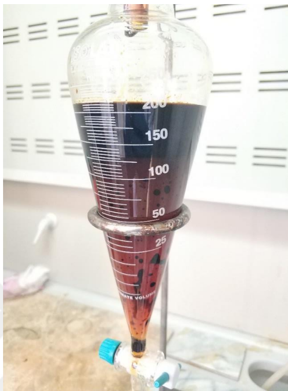
Figure 6.2. Separation of water - bio-oil
