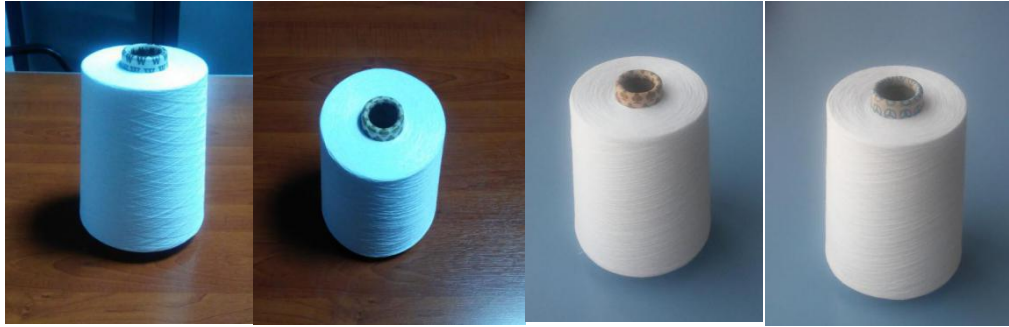
Figure 4.15 Produced %100 pes Ne 20 (oval, blending of scalloped oval and hollow, scalloped oval and hollow cross-section)
