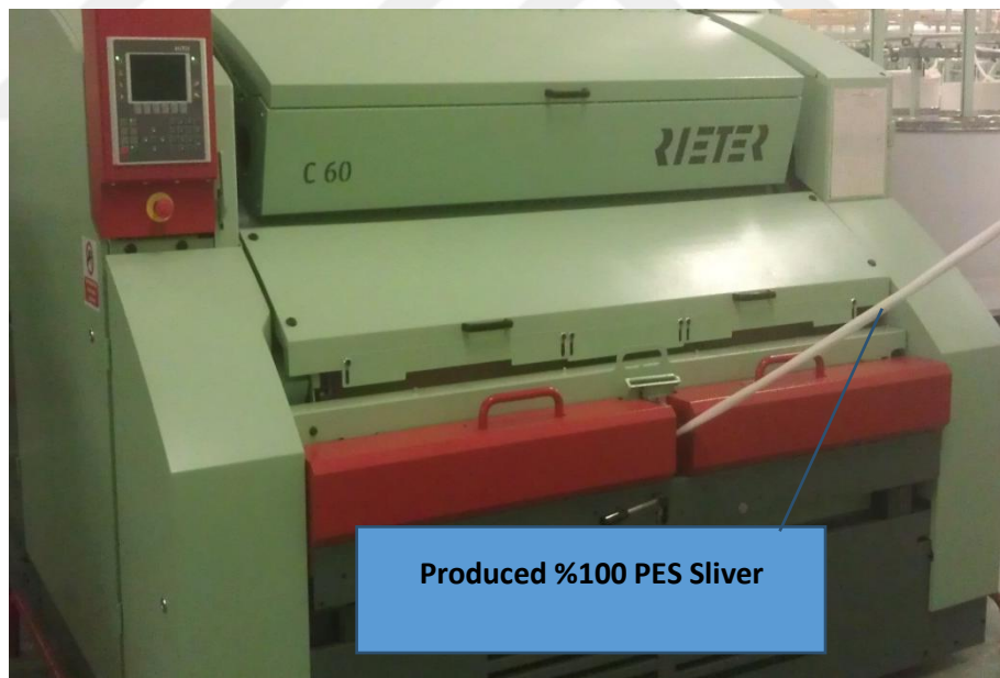
Figure 4.12 Production of carded sliver in carding machine
