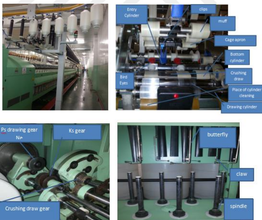
Figure 4.9 Roving frame setting places for fiber
