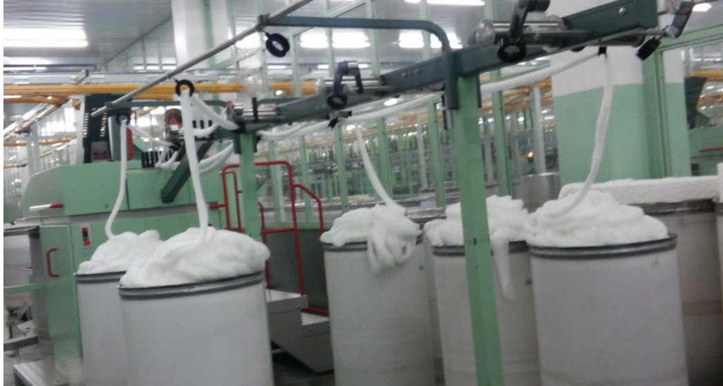
Figure 4.13 Production of polyester sliver with 5-cans at draw frame
