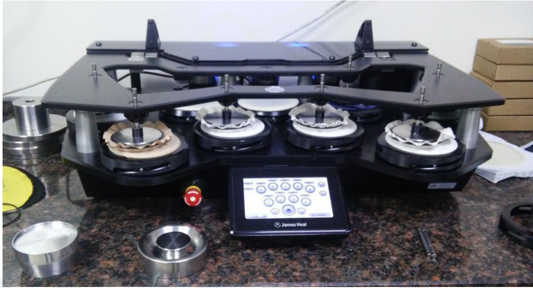
Figure 4.20 The device used for fabrics abrasion resistance test ( James H. Heal martindale abrasion tester )
