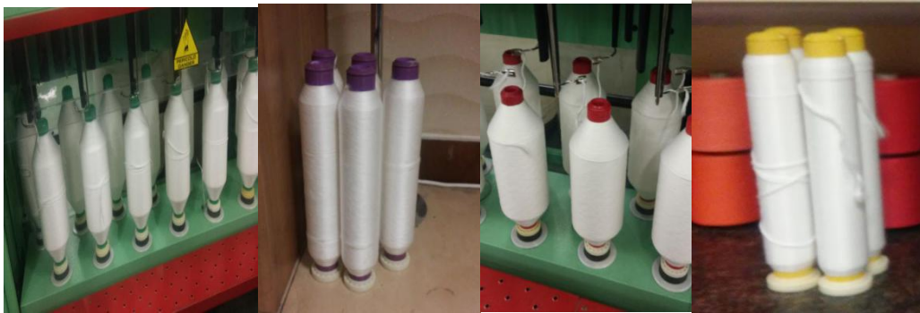
Figure 4.14 Production of pes roving(oval, blending of scalloped oval and hollow, scalloped oval and hollow cross-section) at roving frame
