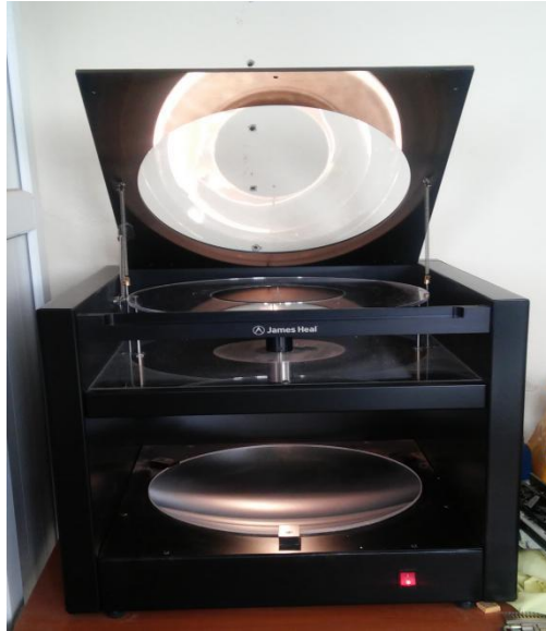
Figure 4.22 The device used for fabrics drape test ( James Heal Drape Tester )
