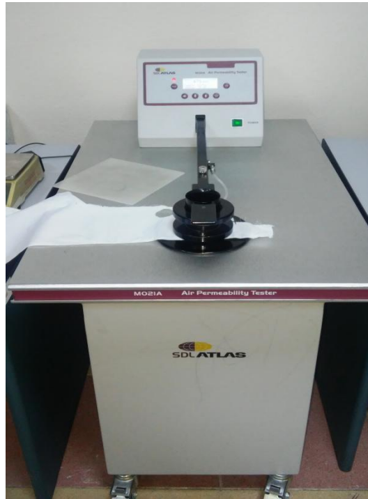
Figure 4.21 The device used for fabrics air permeability test (SDL ATLAS air permeability tester)
