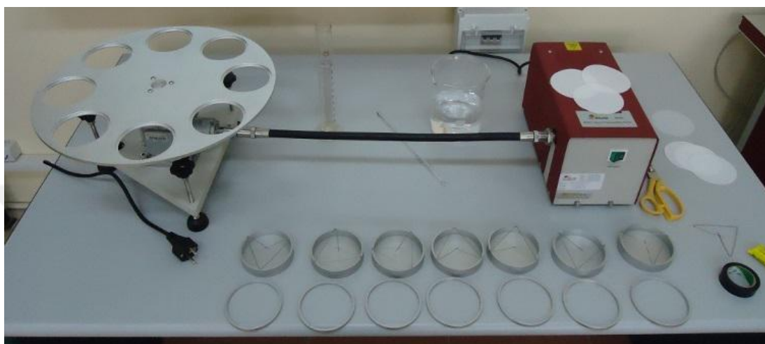
Figure 4.25 The device used for fabrics water vapor permeability test ( SDL ATLAS water vapor permeability tester )
