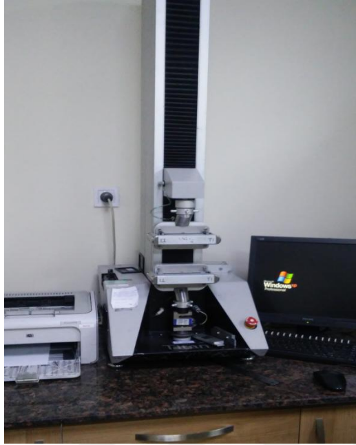
Figure 4.18 The device used for fabrics strength tests ( James H. Heal Titan universal strength tester 2 )
