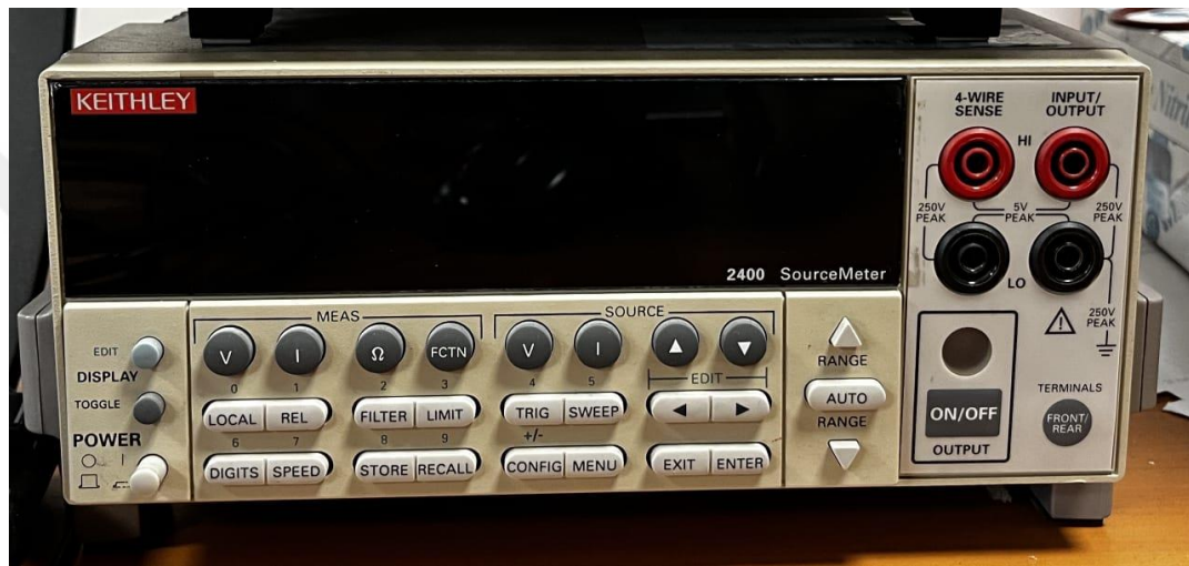
Figure 3.4 Keithley 2400 current-voltage measurement device (Gazi university lab 2023)
