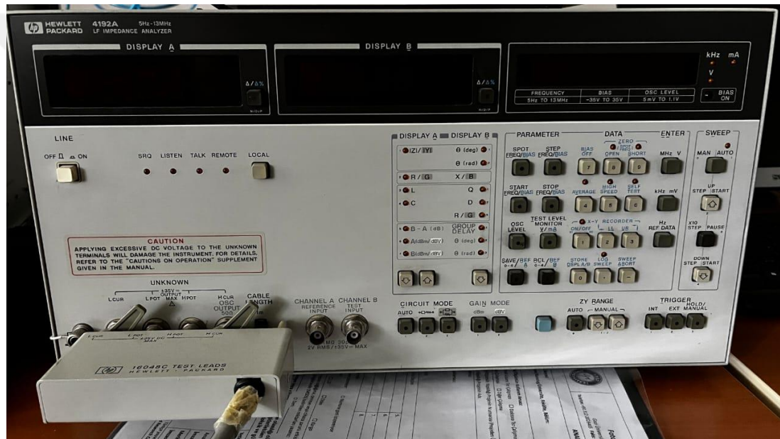
Figure 3.5 Hewlett Packard 4192A LF Impedance Analyzer was utilized to conduct G/\omega -V and C-V measurements on the Au/PVP/n-Si in an experimental setup (Gazi university lab 2023)
