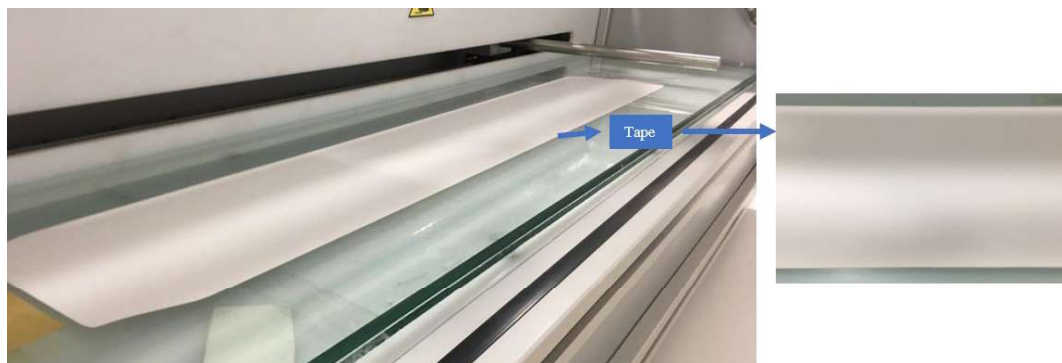
Figure 3.3 Drying process of green tape.
