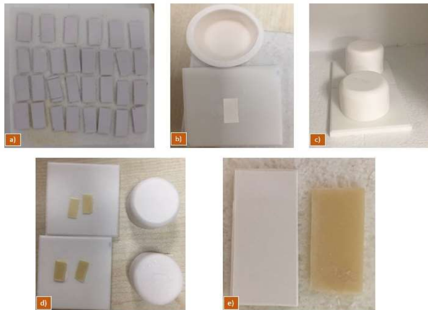
Figure 3.6 Sintering process of 0.68\text{CaTiO}_3\text{-}0.32\text{Ca}(\text{Zn}_{1/3}\text{Nb}_{2/3})\text{O}_3 a) green bodies, b) green bodies on alumina crucible, c) crucible that placed on furnace, d) sintered ceramics on crucible, e) green tape (left) and sintered body (right).
