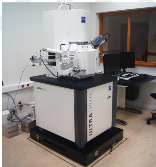
Figure 2.3-3 Zeiss ultra plus field emission Scanning Electron Microscope (SEM)
