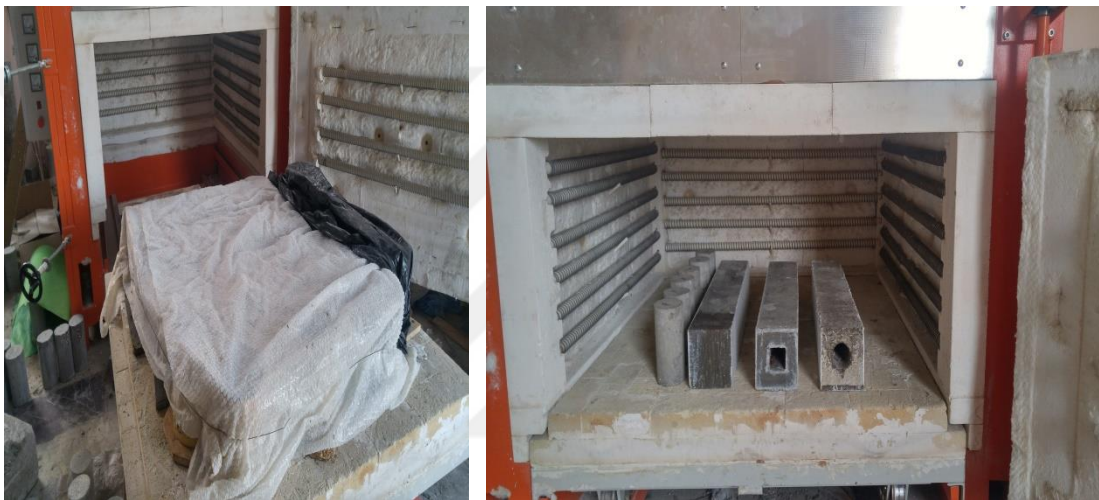
Figure 3.10 The curing of GPC in oven
