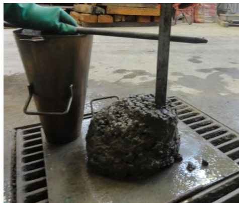
Figure 3.12 Fresh GPC and slump measurement
