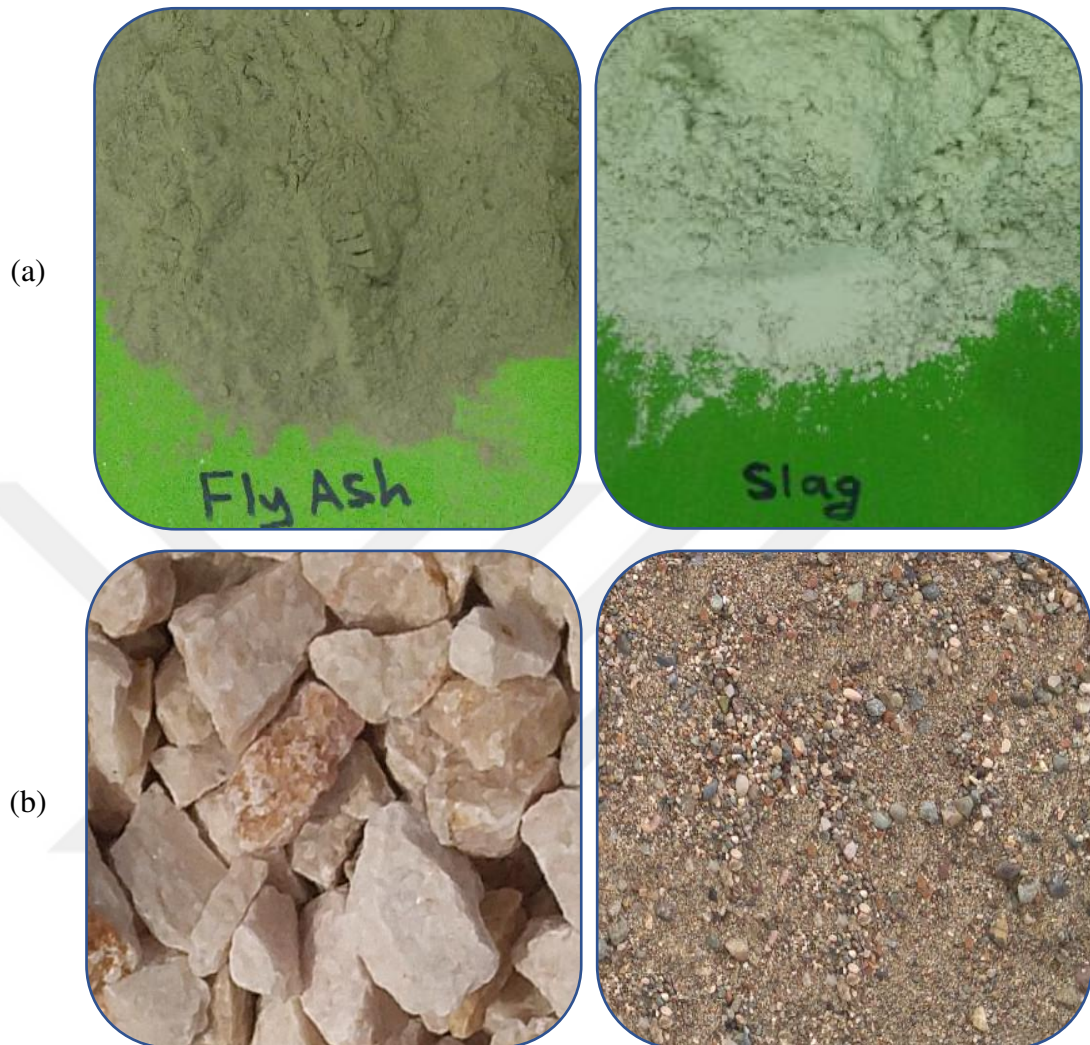
Figure 3.4 (a) Fine materials for matrix (b) Fine and Coarse aggregate
