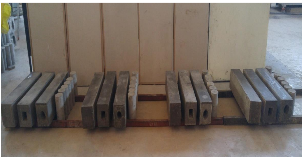
Figure 3.11 Specimens after curing and demoulding
