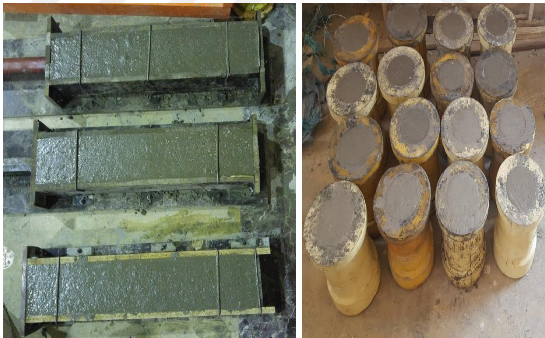
Figure 3.8 Freshly mixed concrete placed in cylinders and beams
