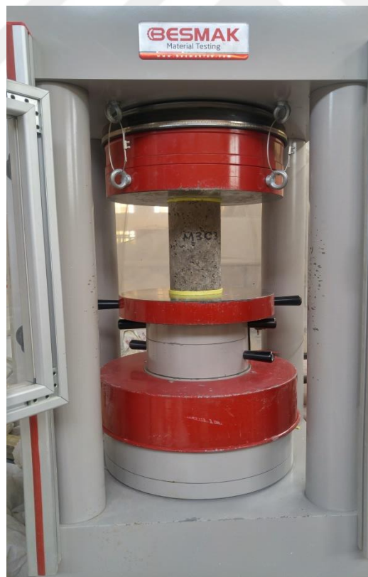
Figure 3.13 Cylinder compressive test
