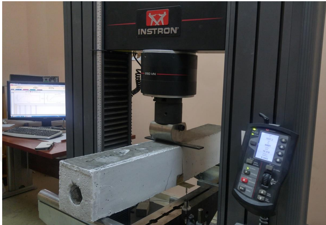
Figure 3.16 Flexural beam test and beam failure
