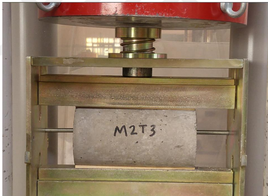
Figure 3.14 Split tensile strength test in progress
