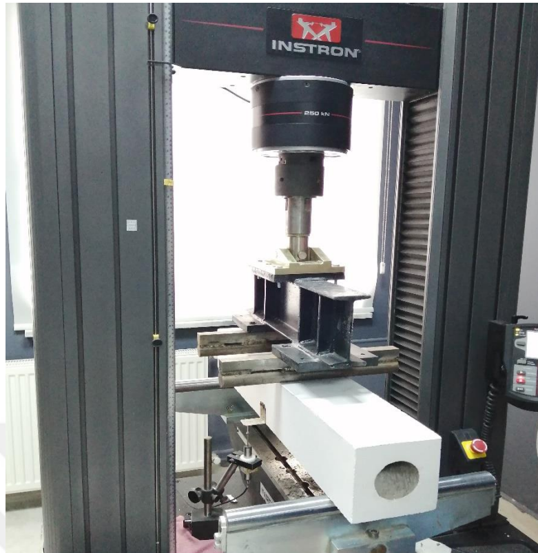
Figure 3.14 Beam test setup.
