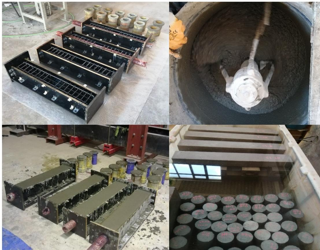
Figure 3.7 Processes of mixing, casting, and curing of specimens.
