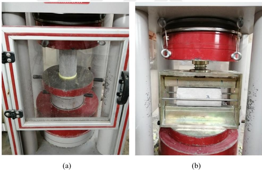
Figure 3.10 Mechanical test (a) compressive strength (b) splitting tensile strength.
