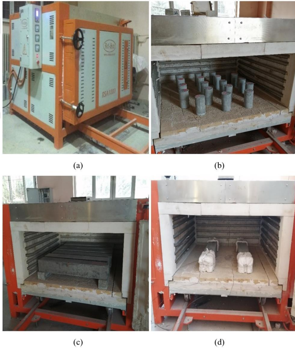
Figure 3.8 Heating process (a) the furnace (b) cylinder specimens drying (c) beams specimens drying (d) beams specimens heating.
