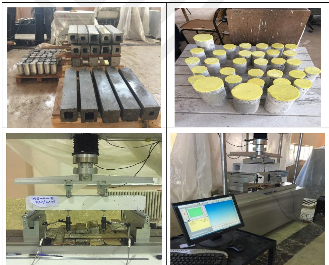
Figure 3.1 Structural elements prior to their test and concrete cylinders
