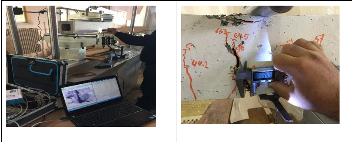
Figure 3.13 The measurement of crack width.
