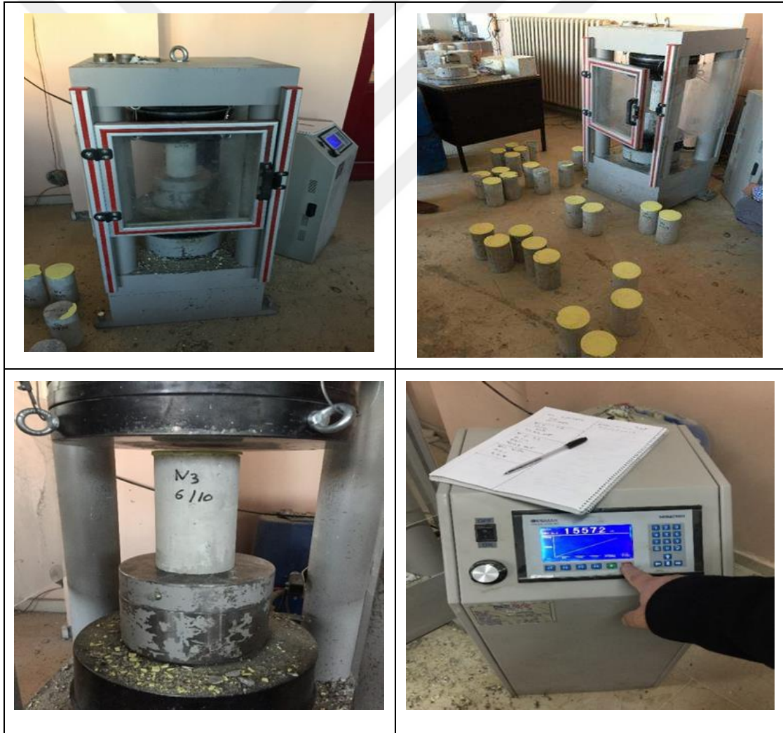
Figure 3.10 The compression strength test setup.
