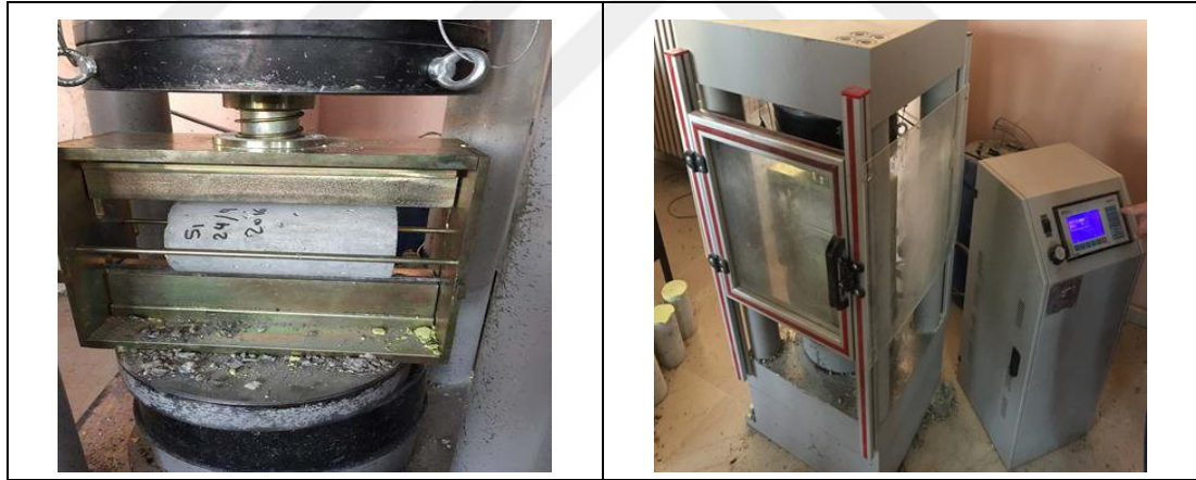
Figure 3.11 Splitting tensile test.
