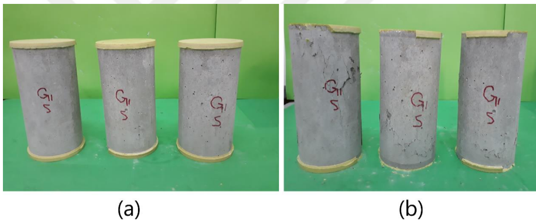
Figure 3.1(a) Specimens before compressive test (b) Specimens after Compressive test
