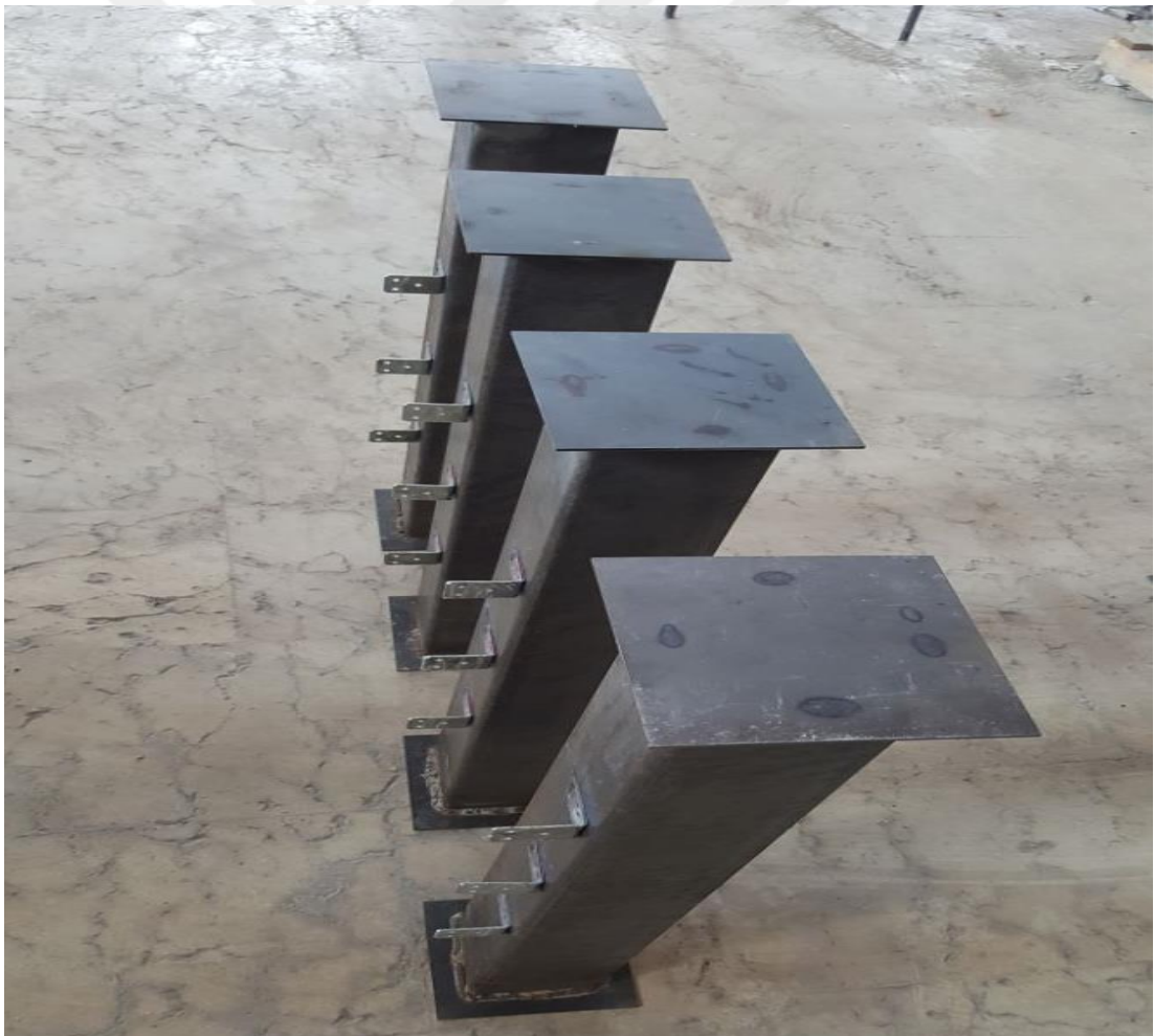
Figure 3.8 The specimens after install steel plate cover
