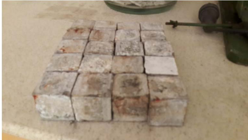
Figure 3.13. The FA Based Geopolymer Concrete Moulds.
