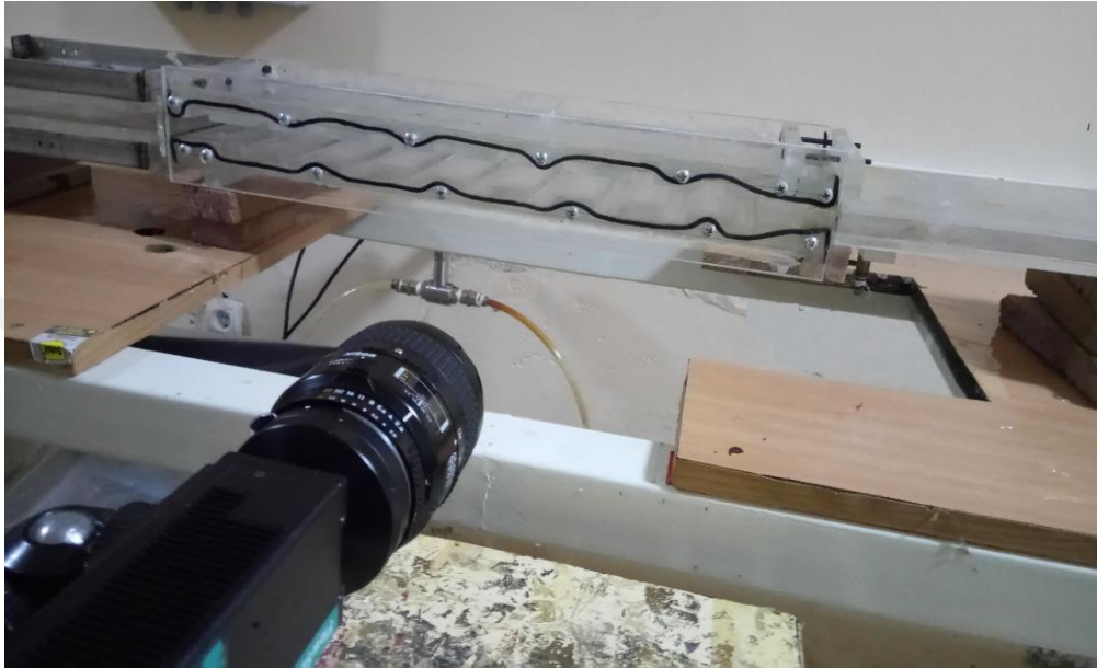
Figure 3.7. The test section made of transparent grooved walls.
