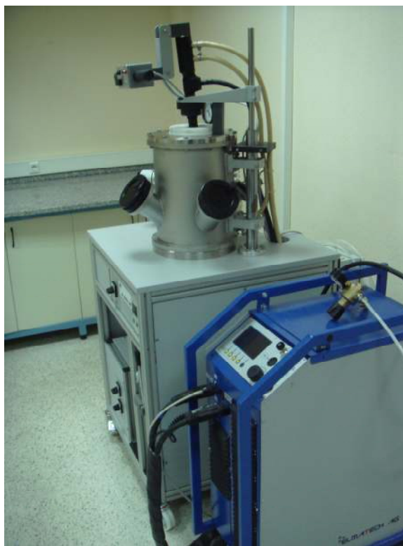
Figure 3.68 Vacuum arc melting equipment.
