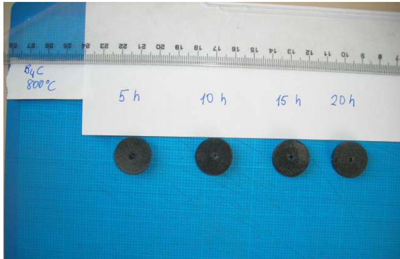
Figure 3.48 B_4C pellets after oxidation at 800^{\circ}C .
