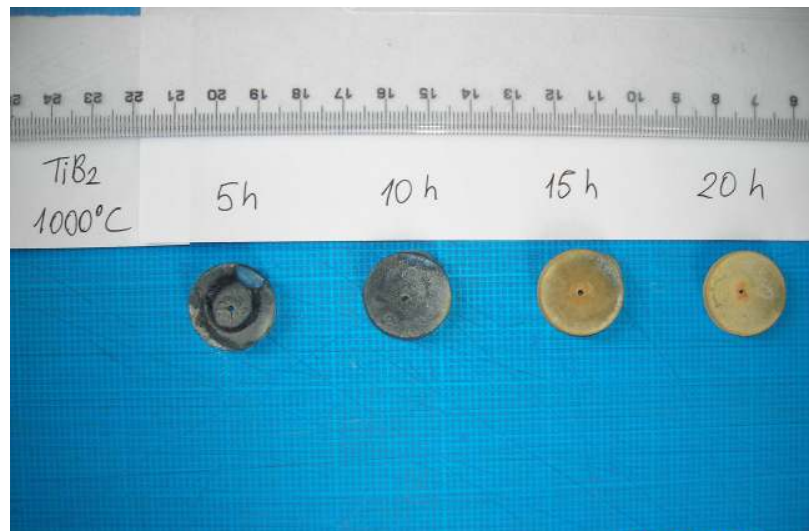
Figure 3.32 TiB 2 pellets after oxidation at 1000°C.
