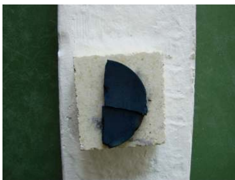
Figure 3.25 \text{TiB}_2 pellet after oxidation at 500°C for 5 hours.
