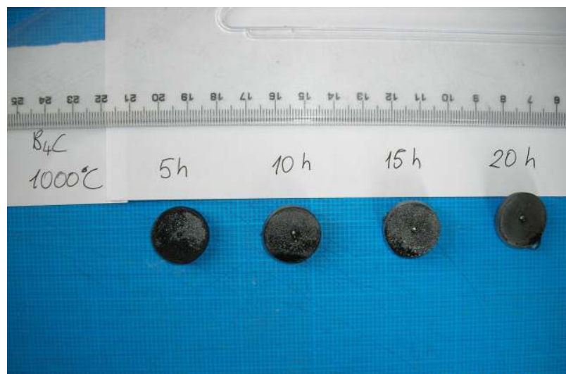
Figure 3.50 B 4 C pellets after oxidation at 1000°C.
