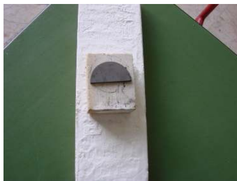
Figure 3.23 The \text{TiB}_2 pellet after oxidation at 300^\circ\text{C} for 4 hours.
