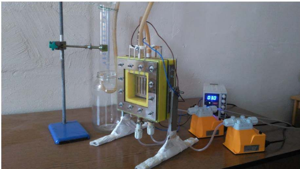
Figure 4.2. Experimental set up producing hydrogen by Chlor-alkali method.
