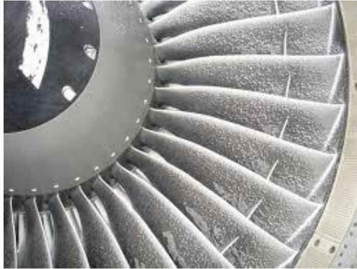
Figure 11. Ice accumulation on engine fan blades [15]
