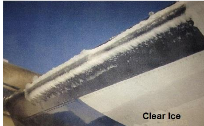
Figure 4. Clear or glaze ice forming around the leading edge of the wing [6]
