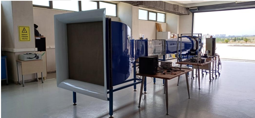
Figure 38. Open suction low-speed wind tunnel for flow visualization and velocity measurement experiments
