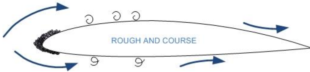
Figure 6. Rime ice accumulation on the surface of the airfoil
