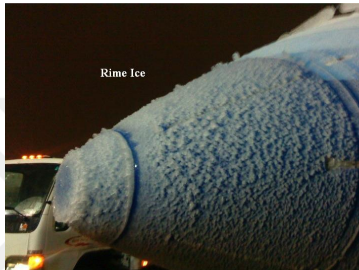
Figure 9. Rime ice accumulated on the fuselage nose [6]
