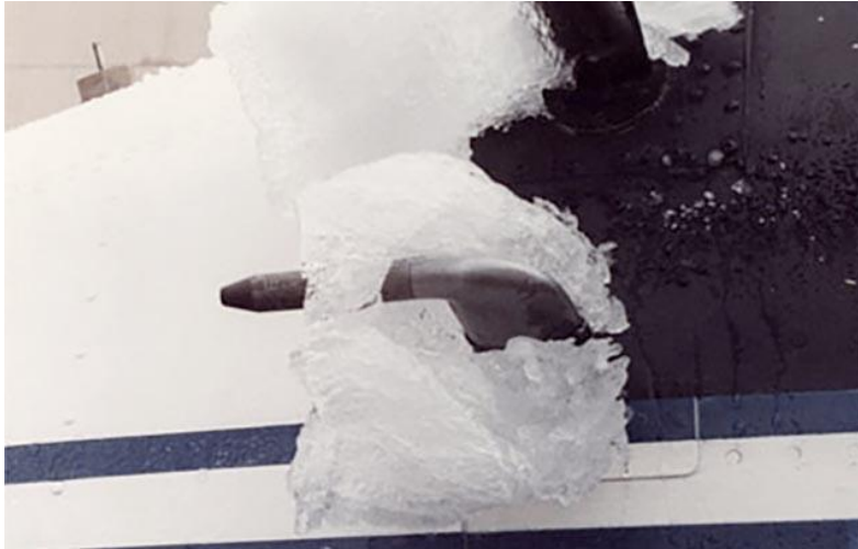
Figure 12. Icing on a Pitot tube [16]
