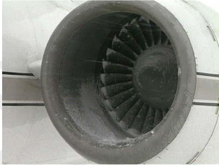
Figure 10. Ice accretion in the engine inlet [13]
