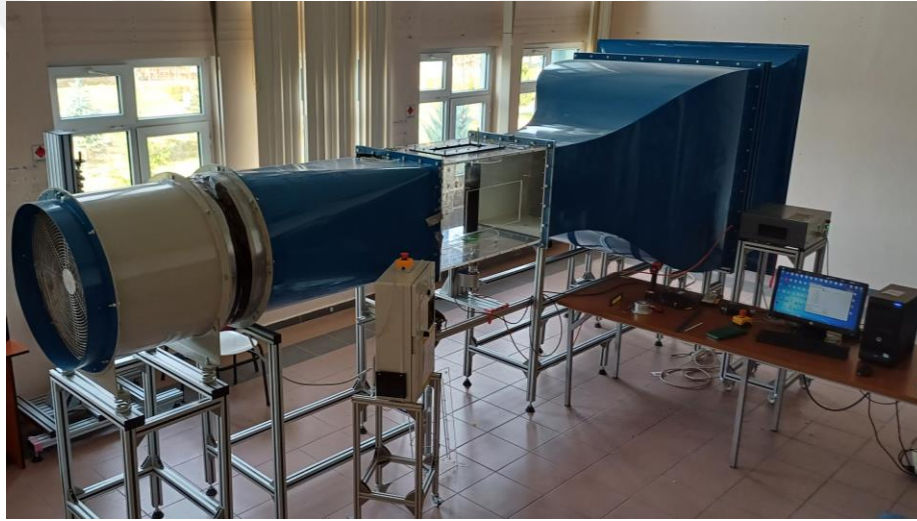
Figure 30. Open suction low-speed wind tunnel in Niğde Ömer Halisdemir University
