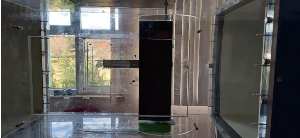
Figure 33. Vertically placed test model in the wind tunnel test section
