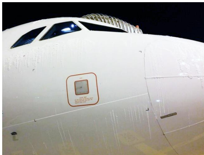
Figure 8. Example of thin ice ridges forward of the pitot probes [11]
