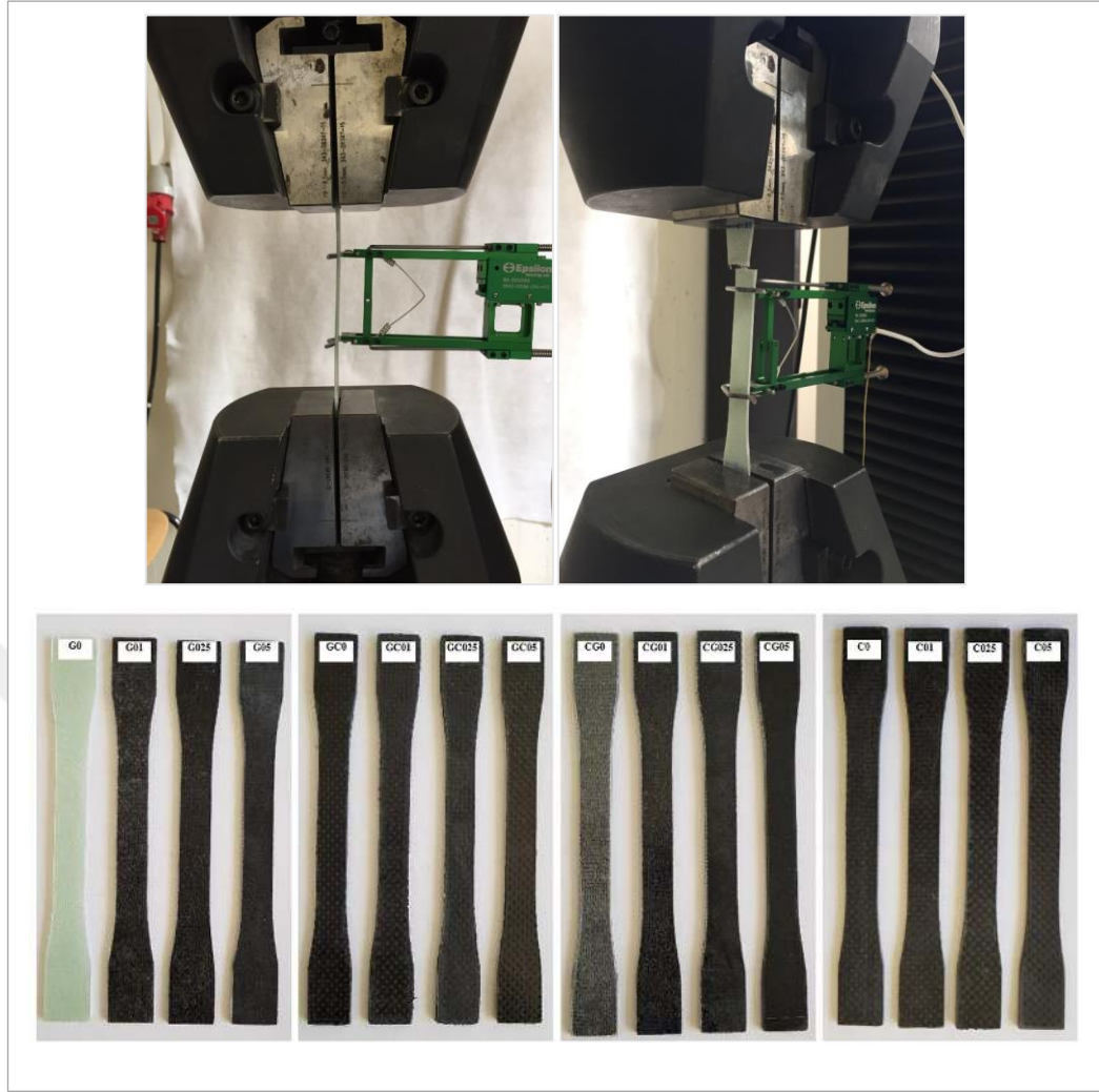
Figure 3.6 Tensile test set-up and test specimens.
