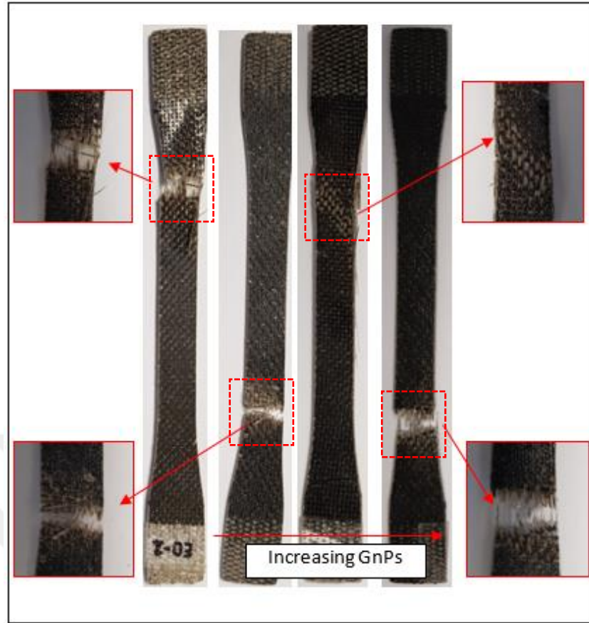
Figure 4.10 Tensile damage figures for BGFR samples with various GnP's content.
