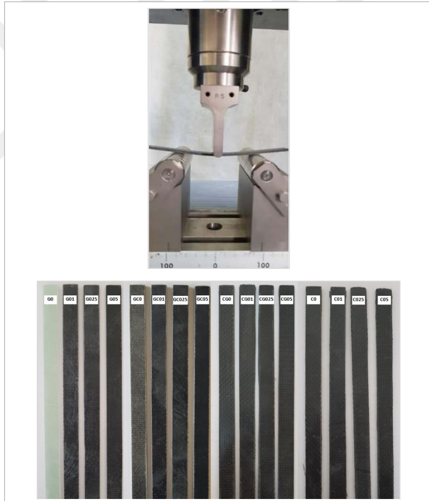
Figure 3.7 Three-point bending test set-up and test specimens.
