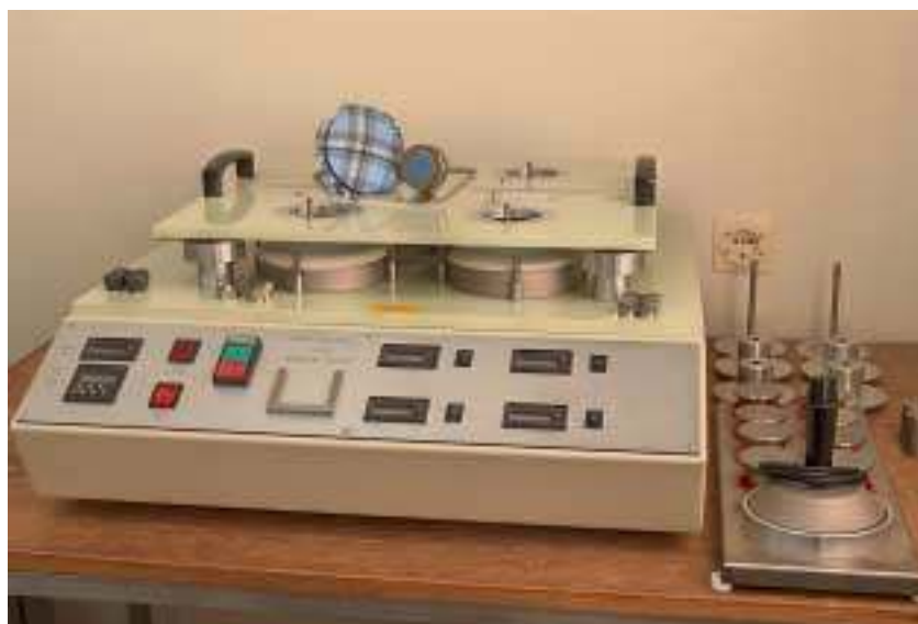
Figure 3. 13 The Martindale Abrasion Tester
