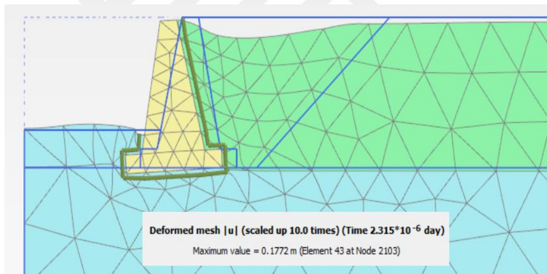
Figure 7.14. Deformed mesh for the second model under dynamic load from Plaxis 2D.
