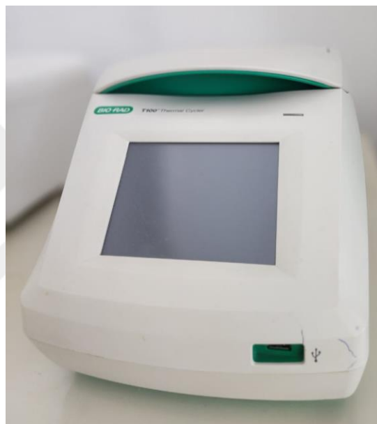
Figure 3.7. PCR Thermal Cycler (Bio-Rad) used in amplification of the LHX4 gene
