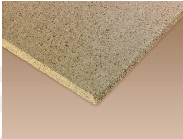
Figure 6.66 Photo of VMT board [285]
