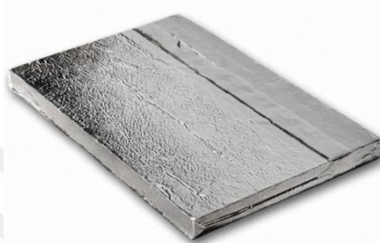
Figure 6.60 Photo of VIP insulation [261]
