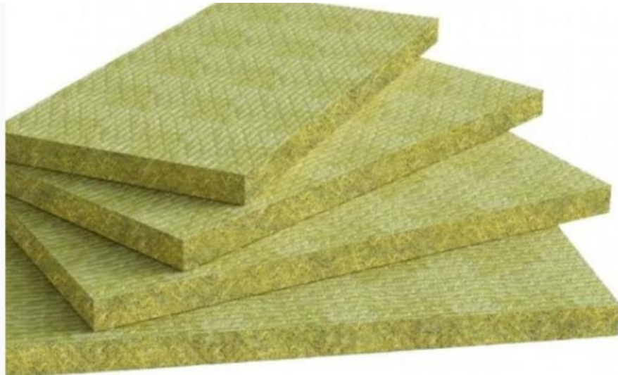
Figure 6.46 Photo of rock wool samples [194]
