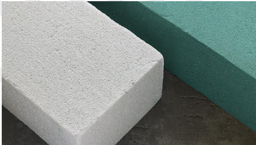
Figure 6.52 Photo of PF samples [220]
