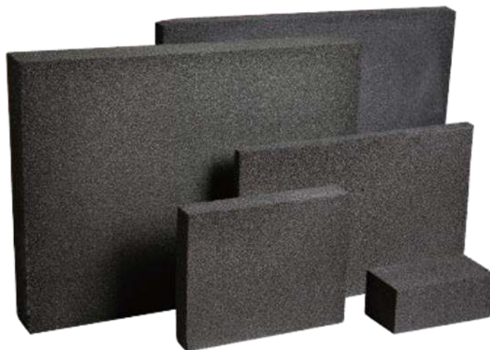
Figure 6.44 Photo of glass foam products [190]
