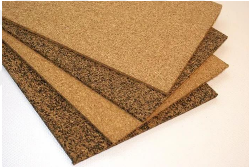
Figure 6.50 Photo of ICB sheets [209]
