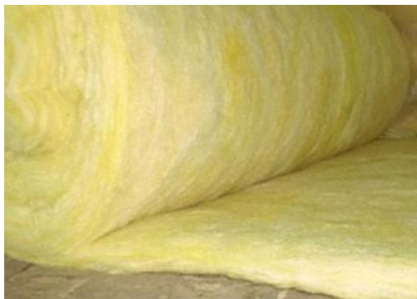
Figure 6.45 Photo of glass wool batt [193]
