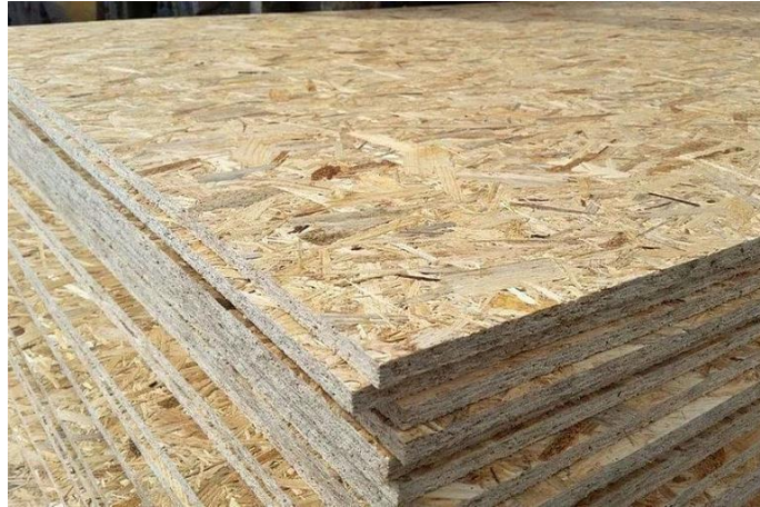
Figure 6.17 Photo of OSB sheets [148]
