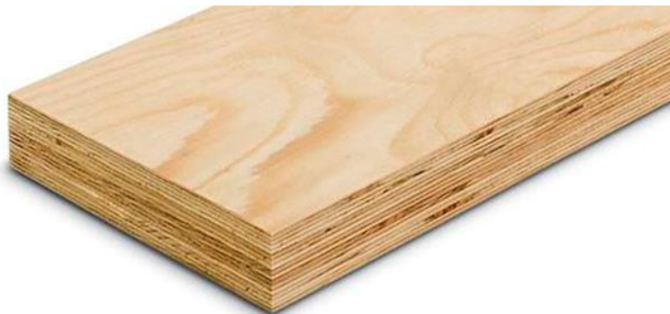
Figure 6.15 Photo of LVL sheet [146]
