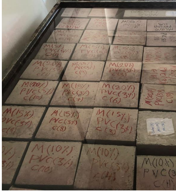
Figure 13: Curing water tank.
