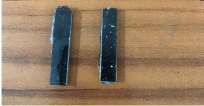
Figure 3.8: Impact test sample according to ISO 179.
