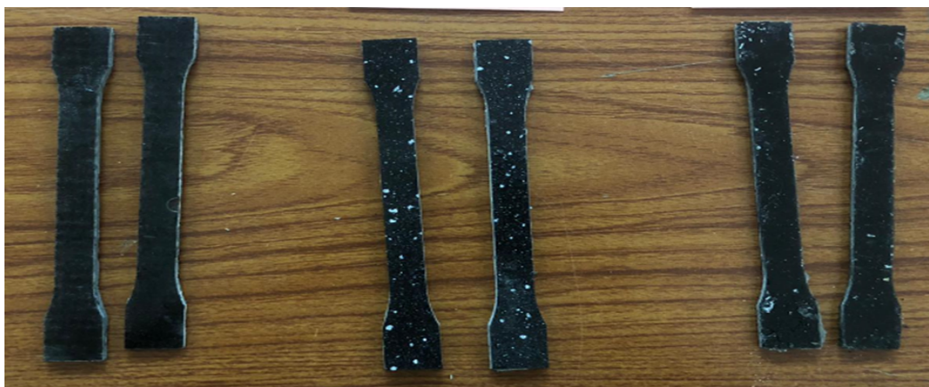
Figure 3.5: Tensile test sample according to ASTM (638M- 78b).
