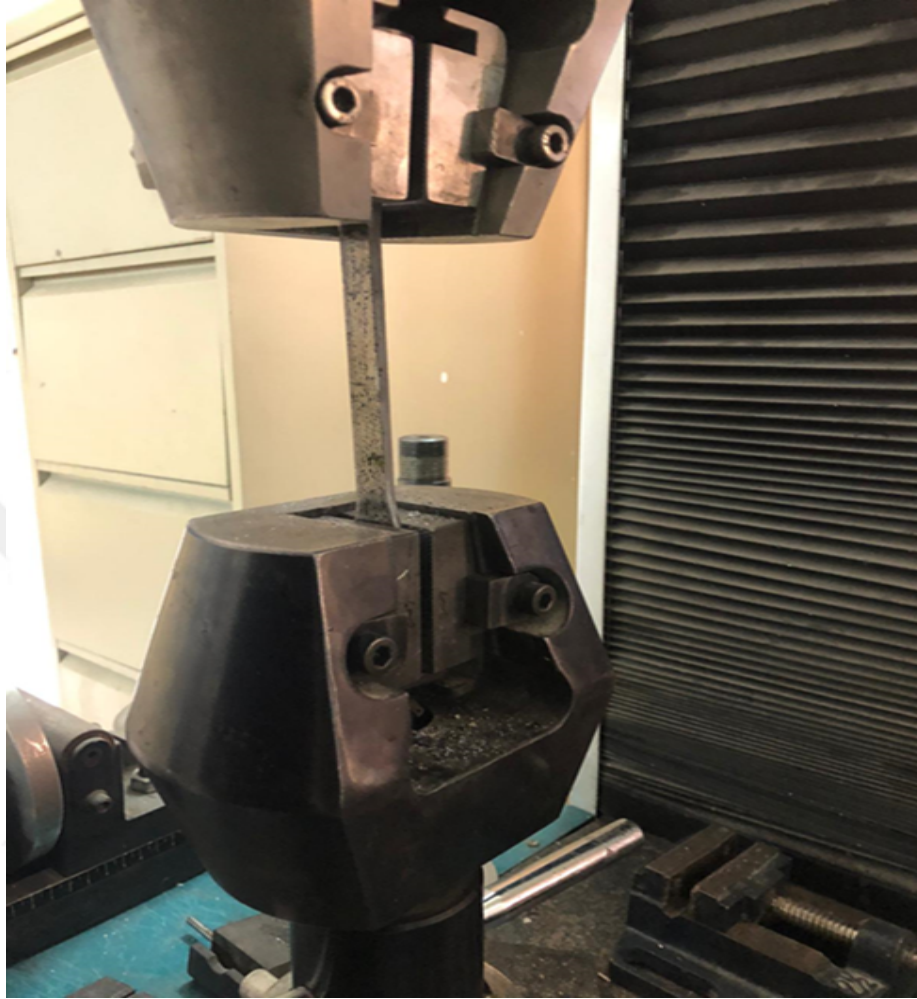
Figure 3.6: Tensile strength test device.
