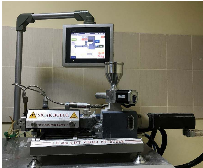
Figure 3.3 Gülnar Makine 12 mm twin screw extruder
