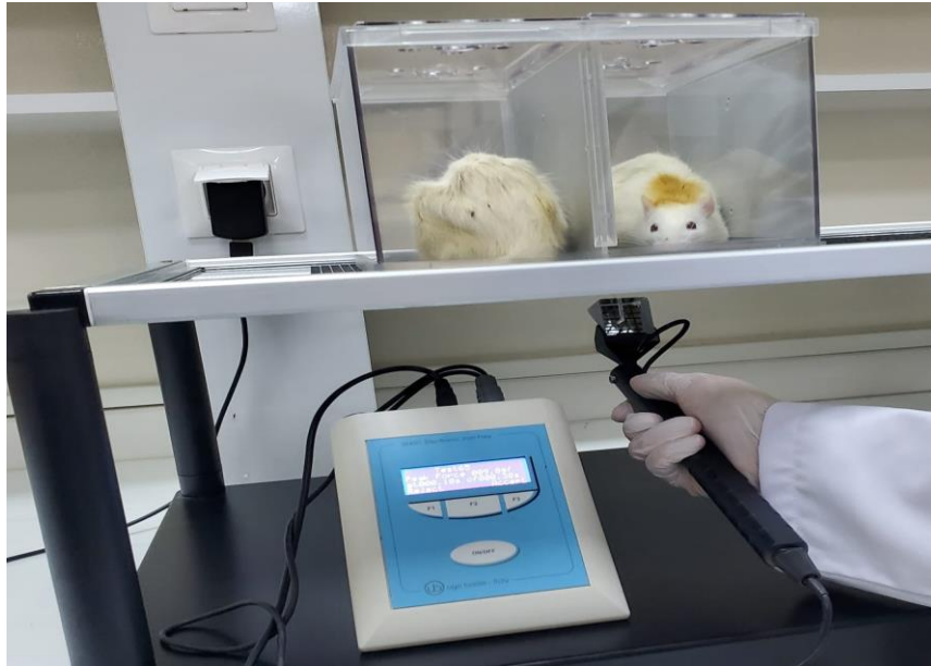
Figure 3.1. E-von Frey apparatus
