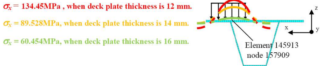
Figure 3.14 Distribution of \sigma_x under wheel load and over rib- web as per deck plate thickness.
