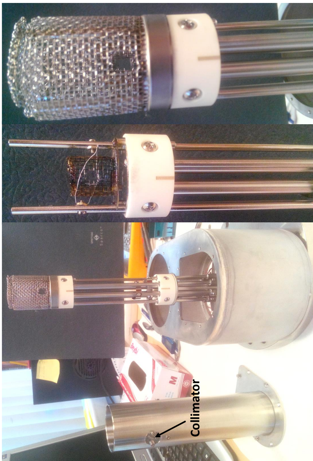
Figure 6.32. Pictures, showing the changes made in DRC and QMS anode grid.
