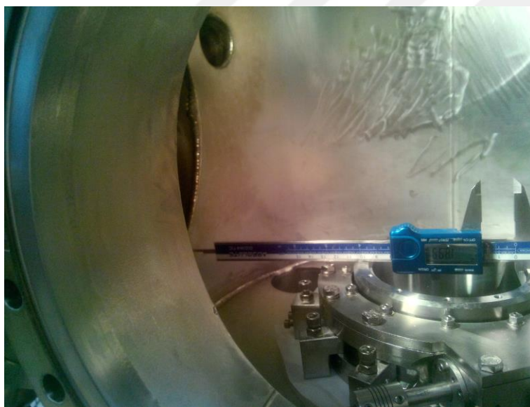
Figure 6.28. Plot showing the alignment of the RP center of rotation with the center of the diffraction chamber.
