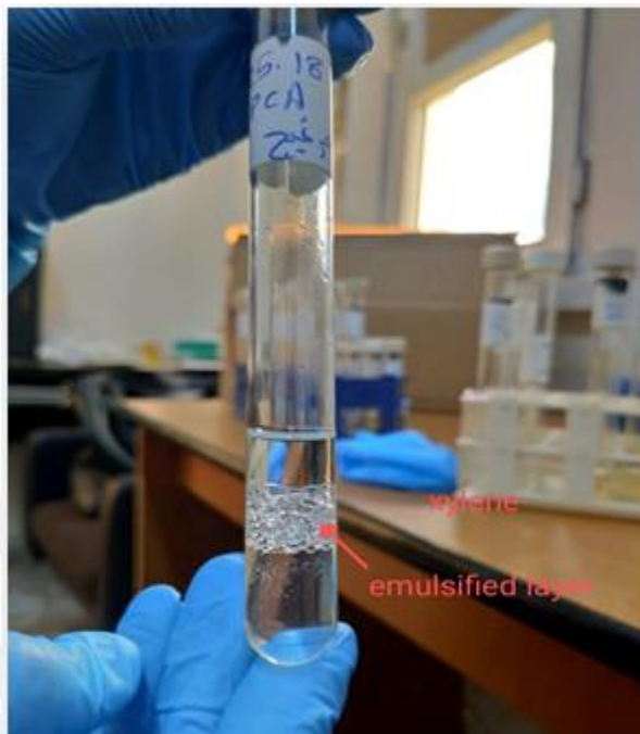
Figure 4.11. Emulsification activity using xylene as hydrocarbon source
