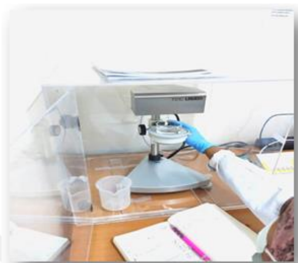
Figure 4.5. Surface tension measurement by using the Optical Contact Angle / Surface Tension Measurement Device (TDIC - LAUDA) and the Ring method
