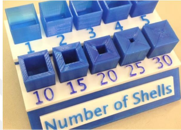
Figure 2.13. The different shell thickness in the same model geometry (Website, 2022b).
