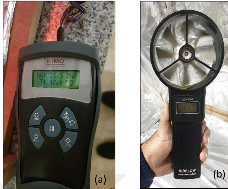
Figure 2. 13 The tools used in experiments (a- Thermometer; b- Airflow meter)
