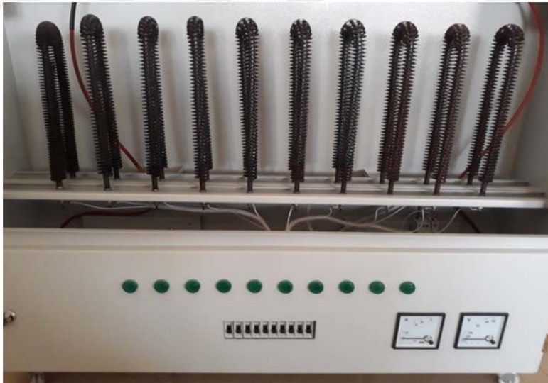
Figure 5.19 . Electric loading system
