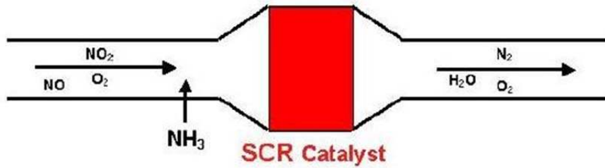
Figure 3.9. Working of SCR (Müller, 2013)
