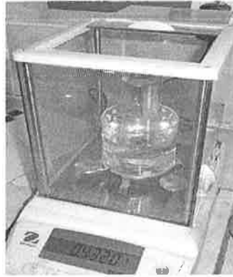
Figure 12. Archimedes density of WPCs
