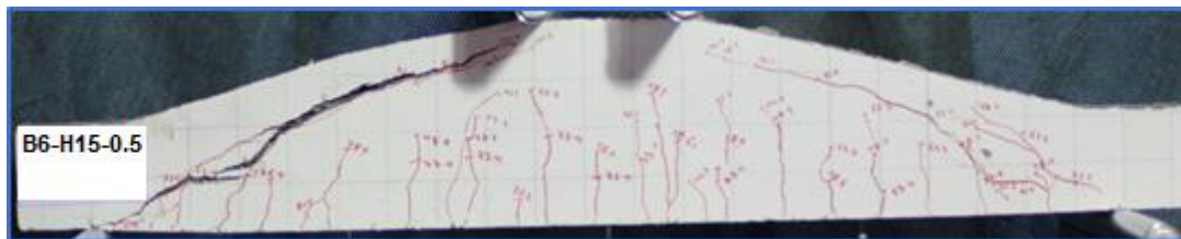
Figure 4.6 Shear Failure for Beam (B6-H15-0.5)
