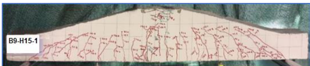
Figure 4.9 Flexural Failure for Beam (B9-H15-1)
