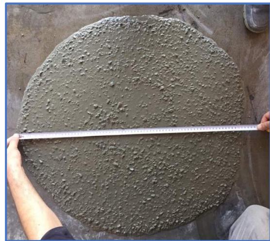
b. The Test of the Slump Flow
