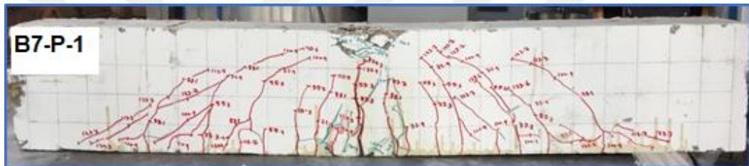
Figure 4.7 Flexural Failure for Beam (B7-P-1)
