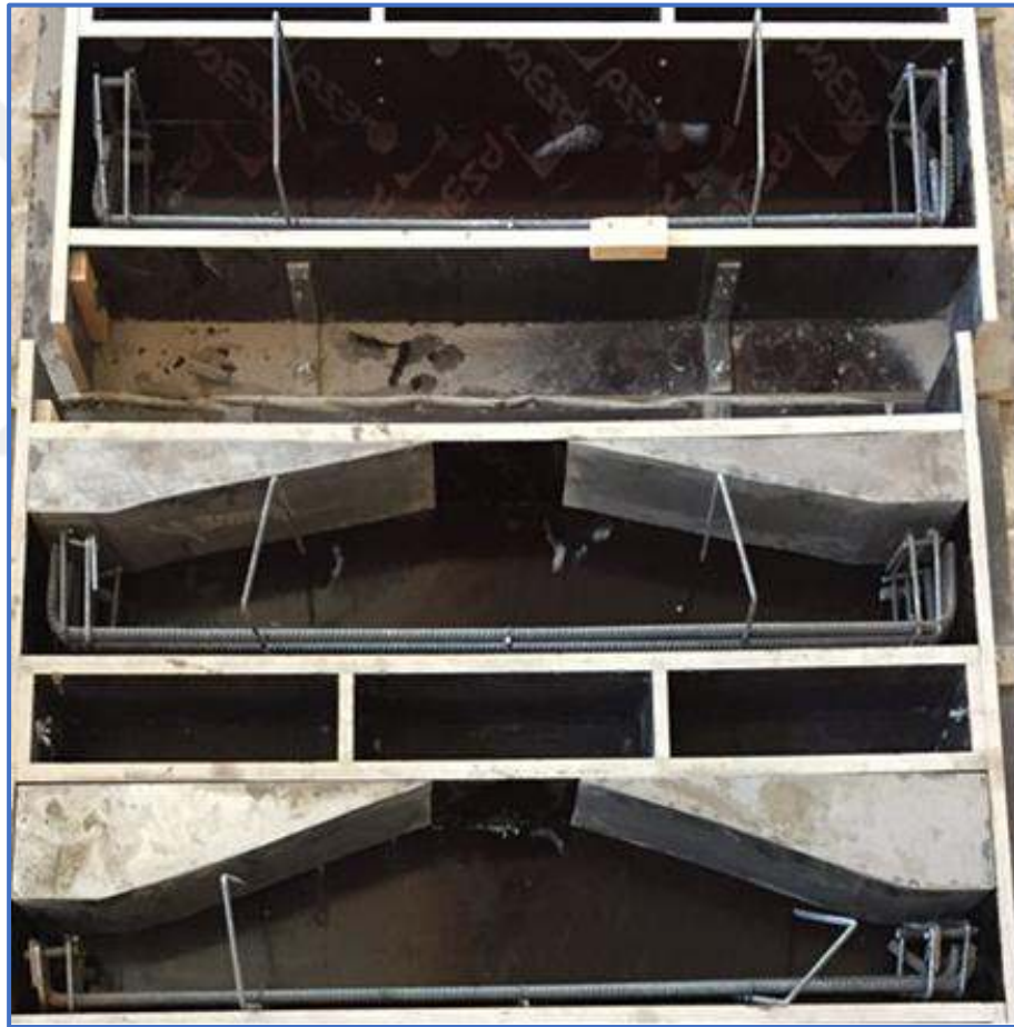
Figure 3.7 Formwork and Reinforcement Configuration for Experimented Beams.
