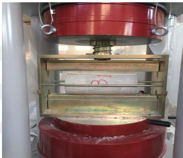
Figure 3.14 Splitting tensile test.
