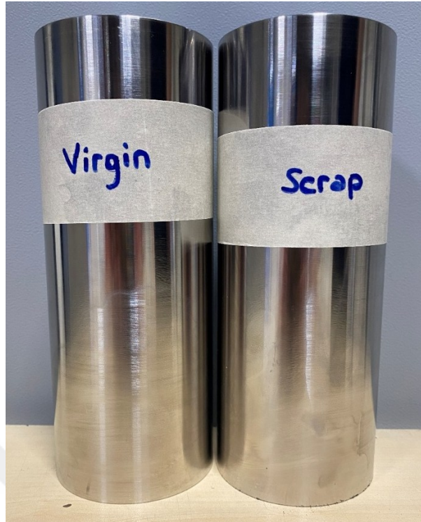
Figure 3.7. Billets with surfaces machined by turning
