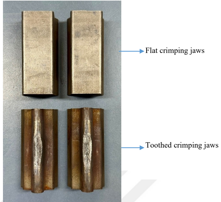
Figure 3.5. Image of the flat and toothed crimping jaws used in the sealing process
