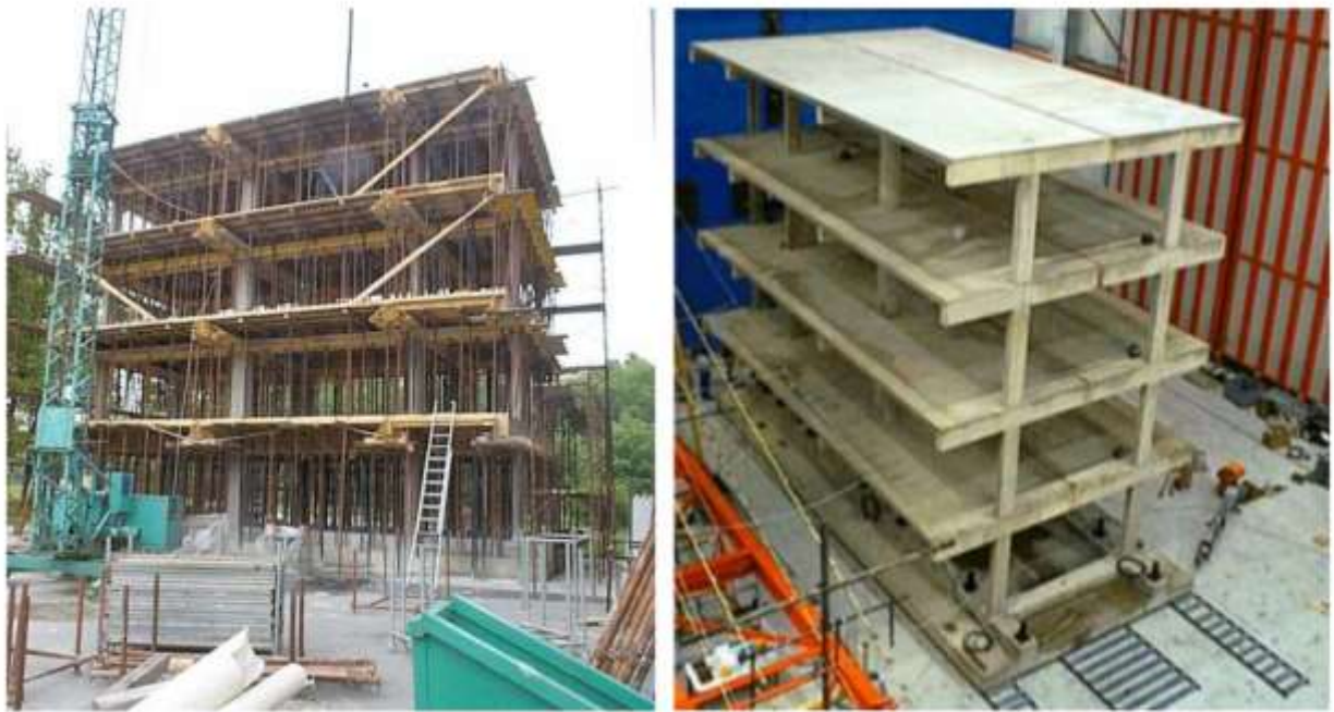
Figure 3.1. Reinforced concrete frame, 4-storey with 3-bays [1].
