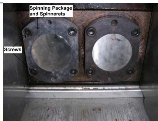
Figure 4.6 Spinning package and spinnerets on the BCF machine
