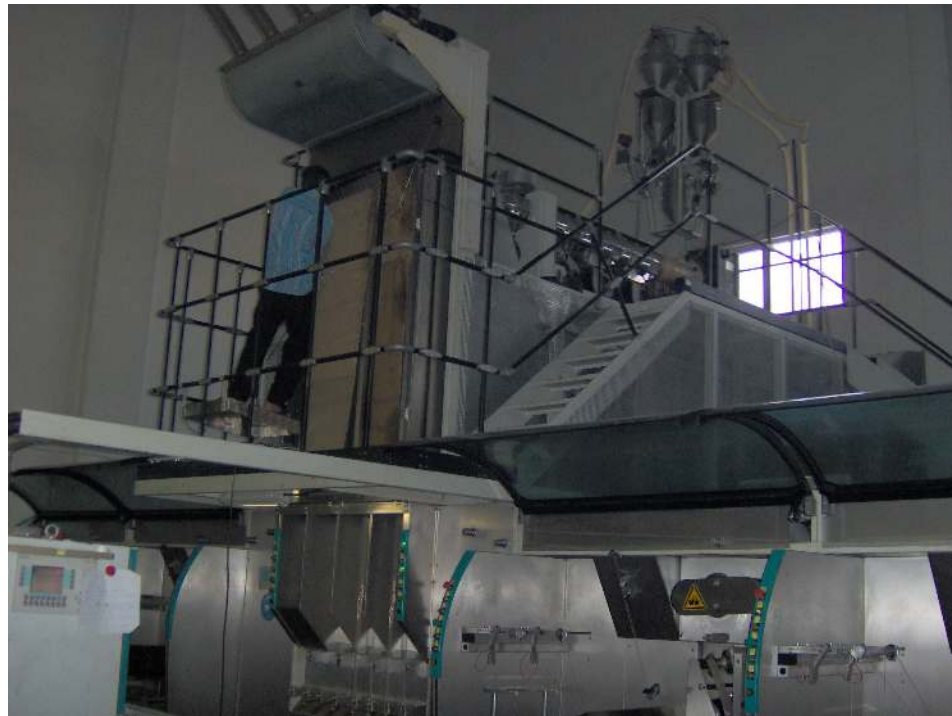
Figure 4.1 The BCF Spinning Machine made by SML
