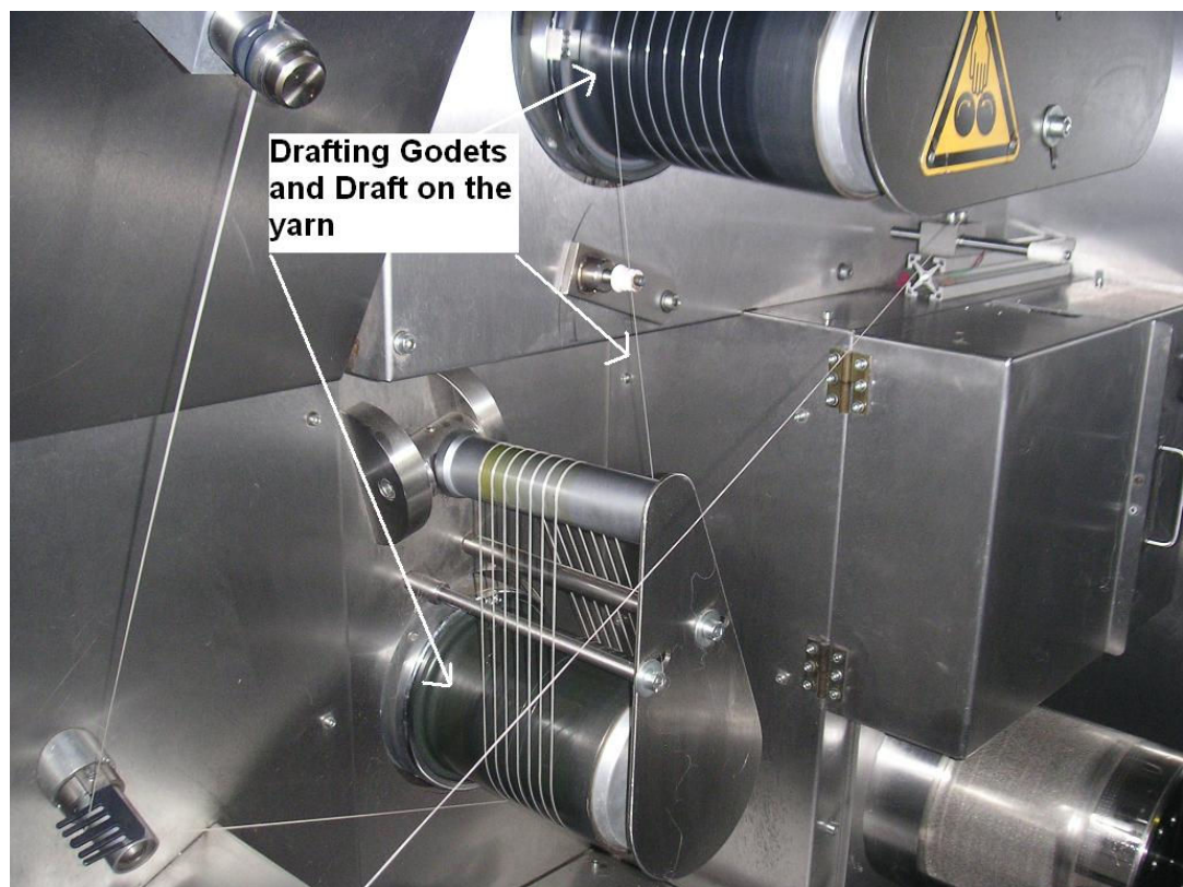
Figure 4.22 The drafting unit drafts the yarn about %3
