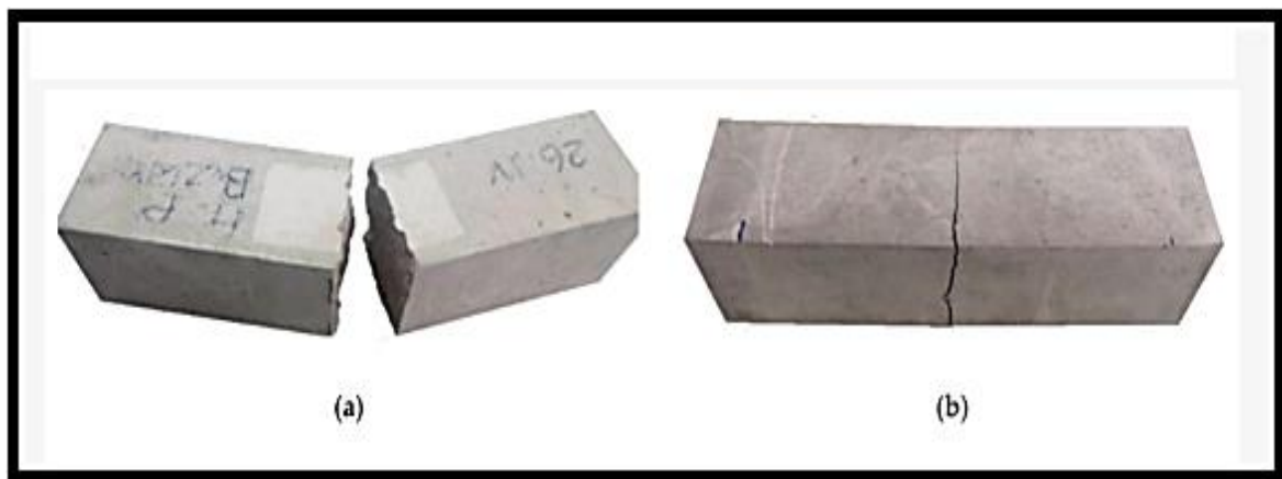
Figure 1.3: Test sample post loading (a) without fiber; (b) with fiber[9]
