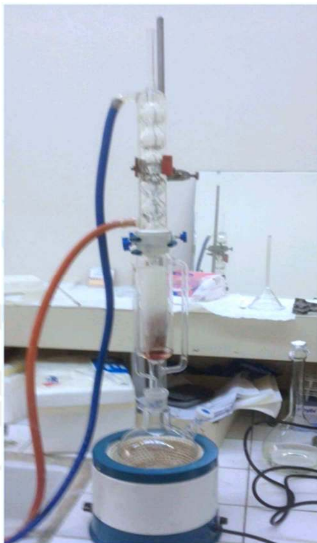
Figure 2.2 Shows the soxhlet extraction setup for the solid-liquid extraction of the samples.
