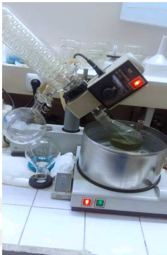
Figure 2.3 Shows the rotary evaporation setup for the extract.
