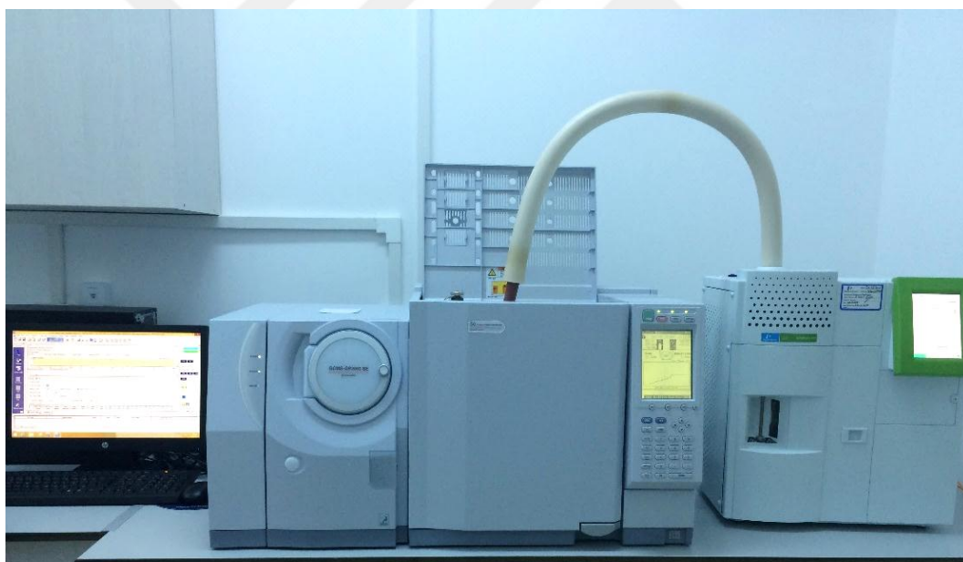
Figure 3.8. TD-GC-MS system used in VOC analysis (photo taken in Environmental Analysis Laboratory in the Chemistry Department of BAIBU).
