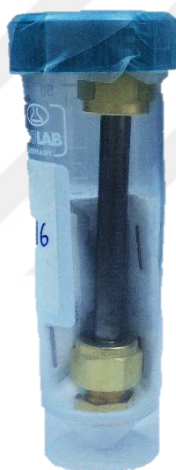
Figure 3.5. Falcon tube including Tenax-TA sampling tube and a pack of silica gel and activated carbon (photo taken in the laboratory).
