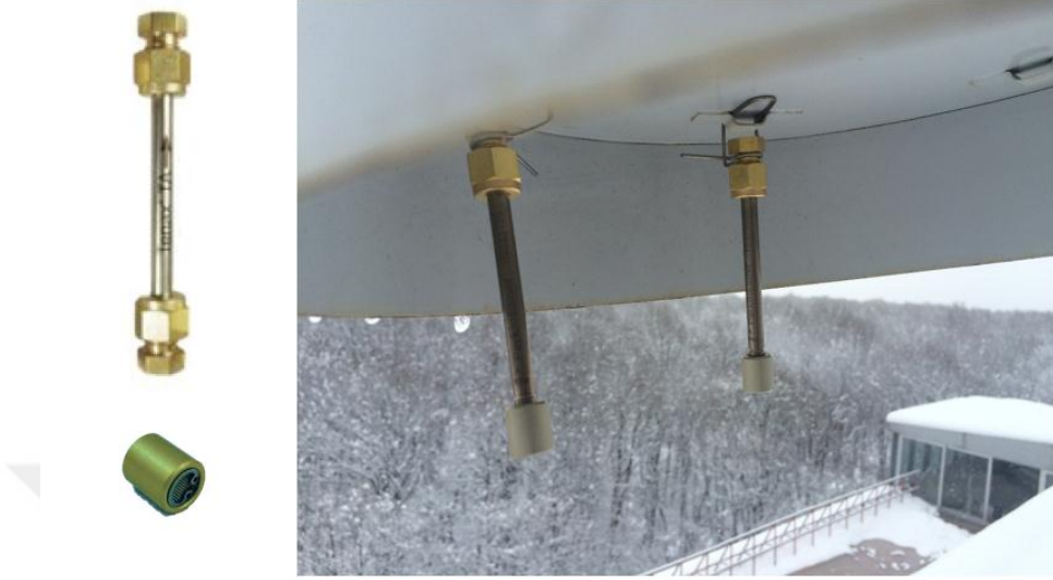
Figure 3.7. Tenax-TA passive sampler connected to the shelter in a sampling area (photo taken in the field).
