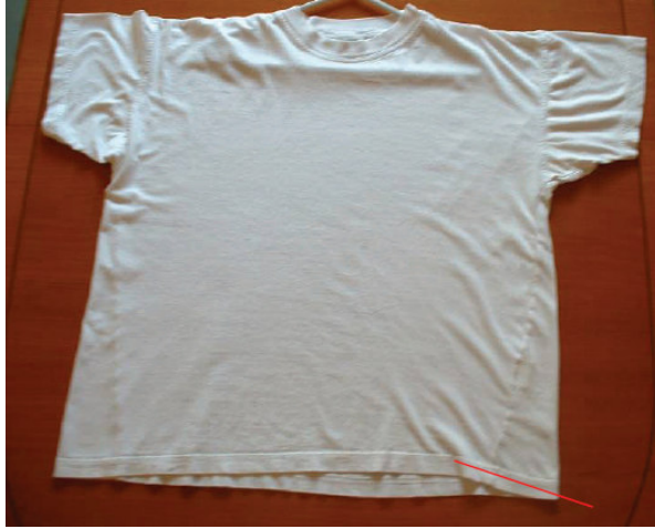
Figure 4.3 Distortion of side seam after laundering
