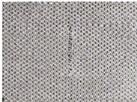
a) Drop stitches on the front side
