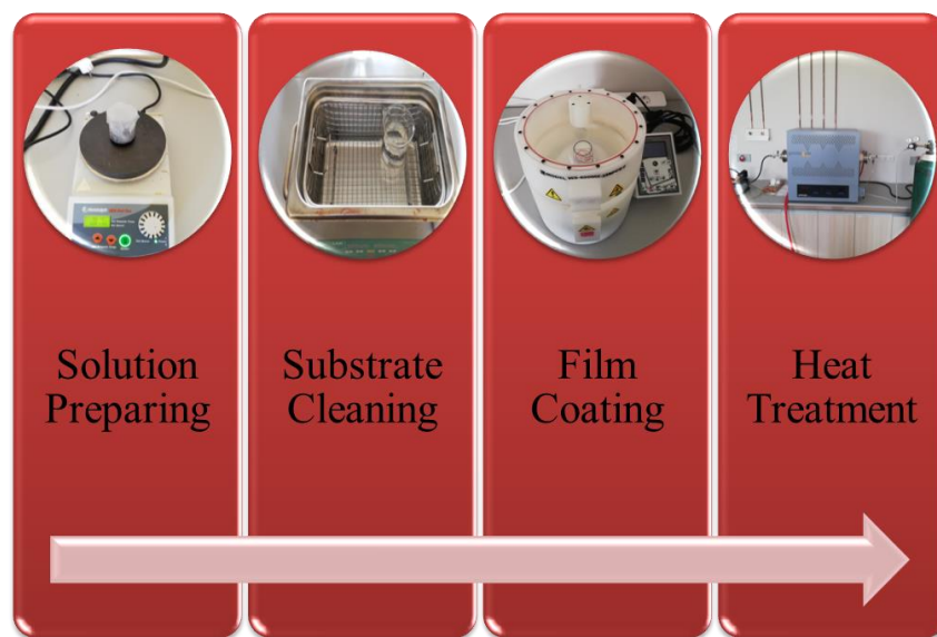
Figure 3.1. Schematic illustration of flow cart of the film manufacturing process.
