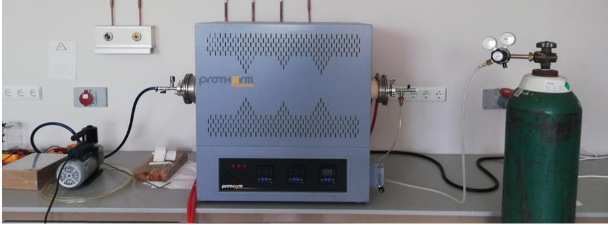
Figure 3.5. The compact system to be carried out heat treatment.
