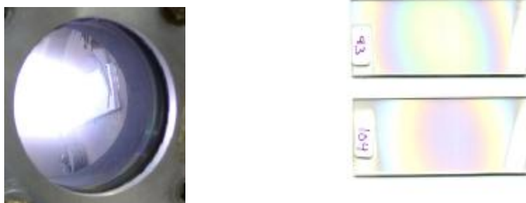
Figure 3.3. Plasma beam impinging onto substrate, and scanned images of two coated substrates.
