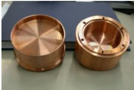
Figure 3.4. Cathodes, showing the cavity for metal filling (left) and water cooling cavity (right).
