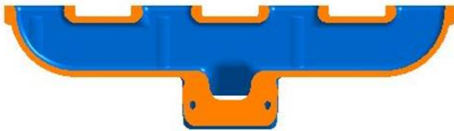
Figure 3.4. Exhaust manifold wall thickness
