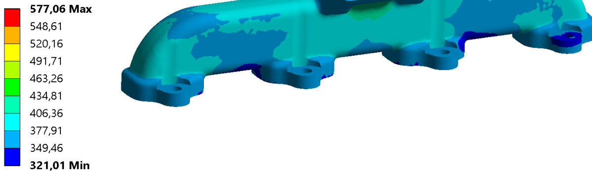
Figure 4.8. Exhaust manifold thermal analysis initial phase
