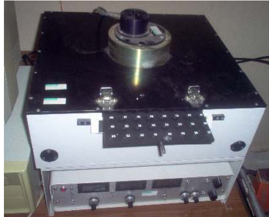
Figure 4.3 9010 Optical Dating System (irradiator)
