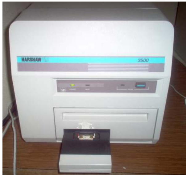
Figure 4.4 Harshaw TLD System 3500 Manual TL Reader
