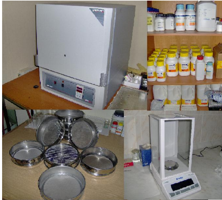
Figure 4.6 Some of the used equipments: oven, chemicals, sieves and digital balance.
