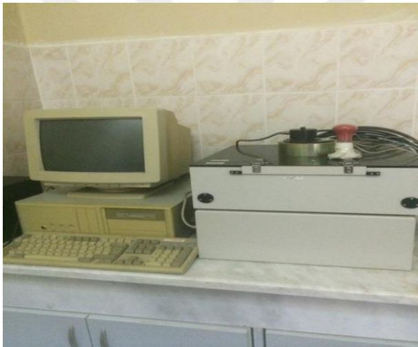
Figure 3.2 Radiation sources of beta ray ^{90}\text{Sr} - ^{90}\text{Y} source ( \approx 0.04\text{Gy/s} ).
