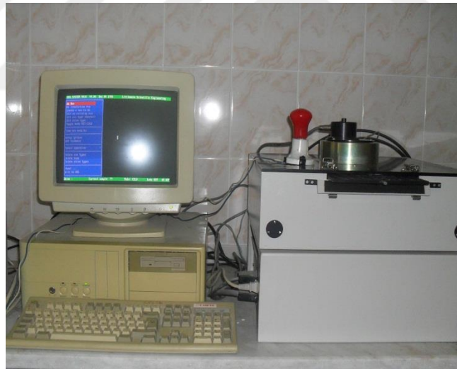
Figure 4.2. ^{90}\text{Sr} - ^{90}\text{Y} \beta - radiation source and 9010 Optical Dating System (irradiator).
