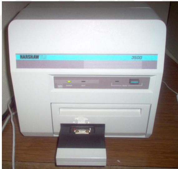
Figure 3.4 Harshaw TLD System 3500 Manual TL Reader.
