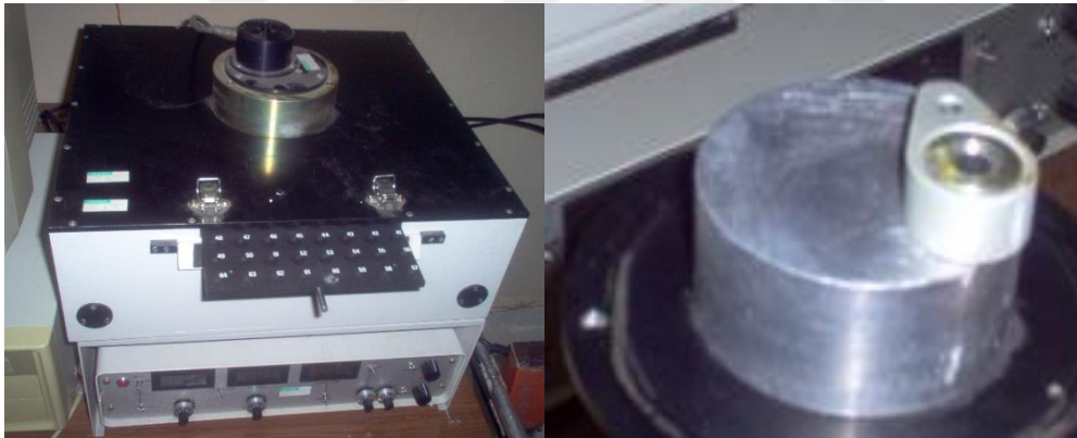
Figure 3.2 9010 Optic Dating System and ^{90}\text{Sr} - ^{90}\text{Y} \beta -source supplementary on it [18].
