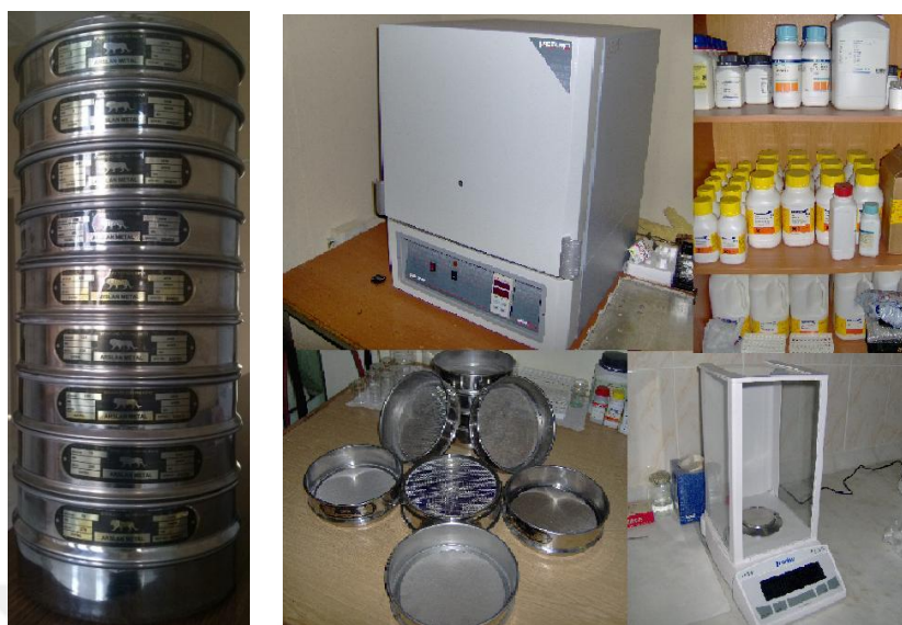
Figure 4.5 Some of the used equipments: oven, chemicals, sieves and digital balance.
