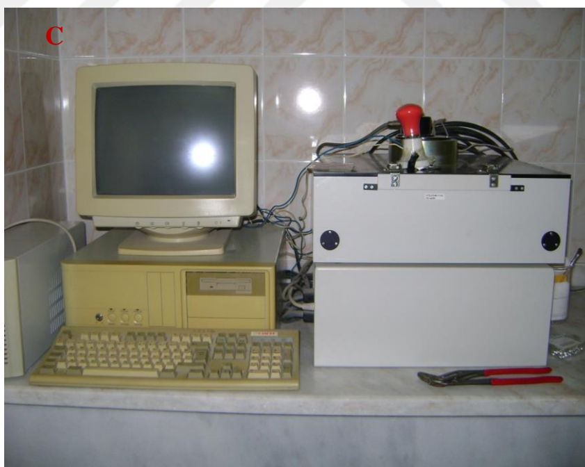
Figure 4.4 ^{90}\text{Sr} - ^{90}\text{Y} \beta radiation source and computer.
