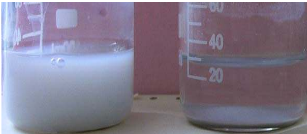
Figure 4.1 Comparative samples showing the alumina nanofluids without and with sedimentation.
