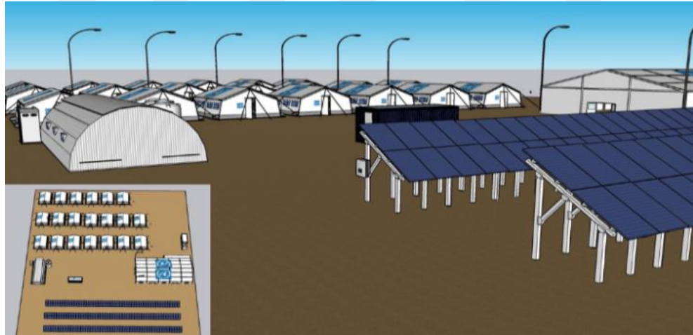
Figure 4.7. 3D drawing of habitat and PV plant.
